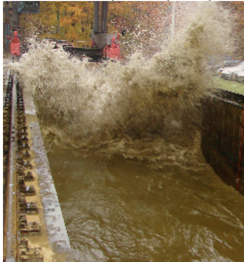
Figure 1.2 Impact of incoming and outgoing (reflected) waves in Deltaflume
