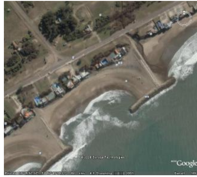
Figure 34 T-head groynes at Longbranch-Bradley beach, North-Atlantic coast, USA (left). T-head and L-head groynes at South-Atlantic coast, Miramar, Argentina (right)
