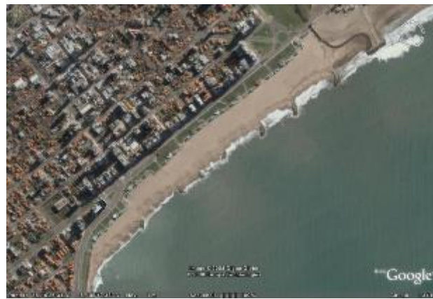
Figure 31 Example of effective groyne design (small compartments) at Miramar beach, Argentina (beach sediments 0.3 to 0.6 mm; ratio of spacing and length \leq 1 to 1.5; crest at +3 m above MSL)
