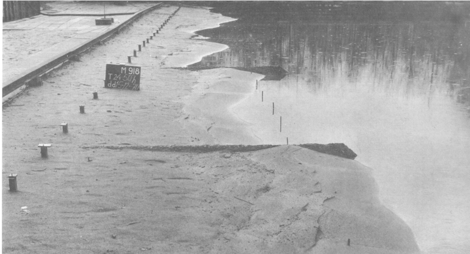
Figure 28 Effect of three groynes on coast, Test T24 (Hulsbergen et al., 1977)
