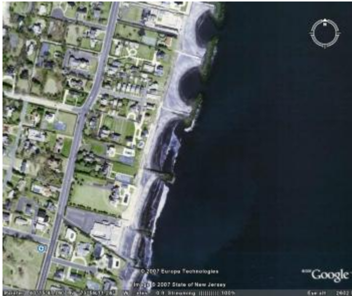
Figure 34 T-head groynes at Longbranch-Bradley beach, North-Atlantic coast, USA (left). T-head and L-head groynes at South-Atlantic coast, Miramar, Argentina (right)
