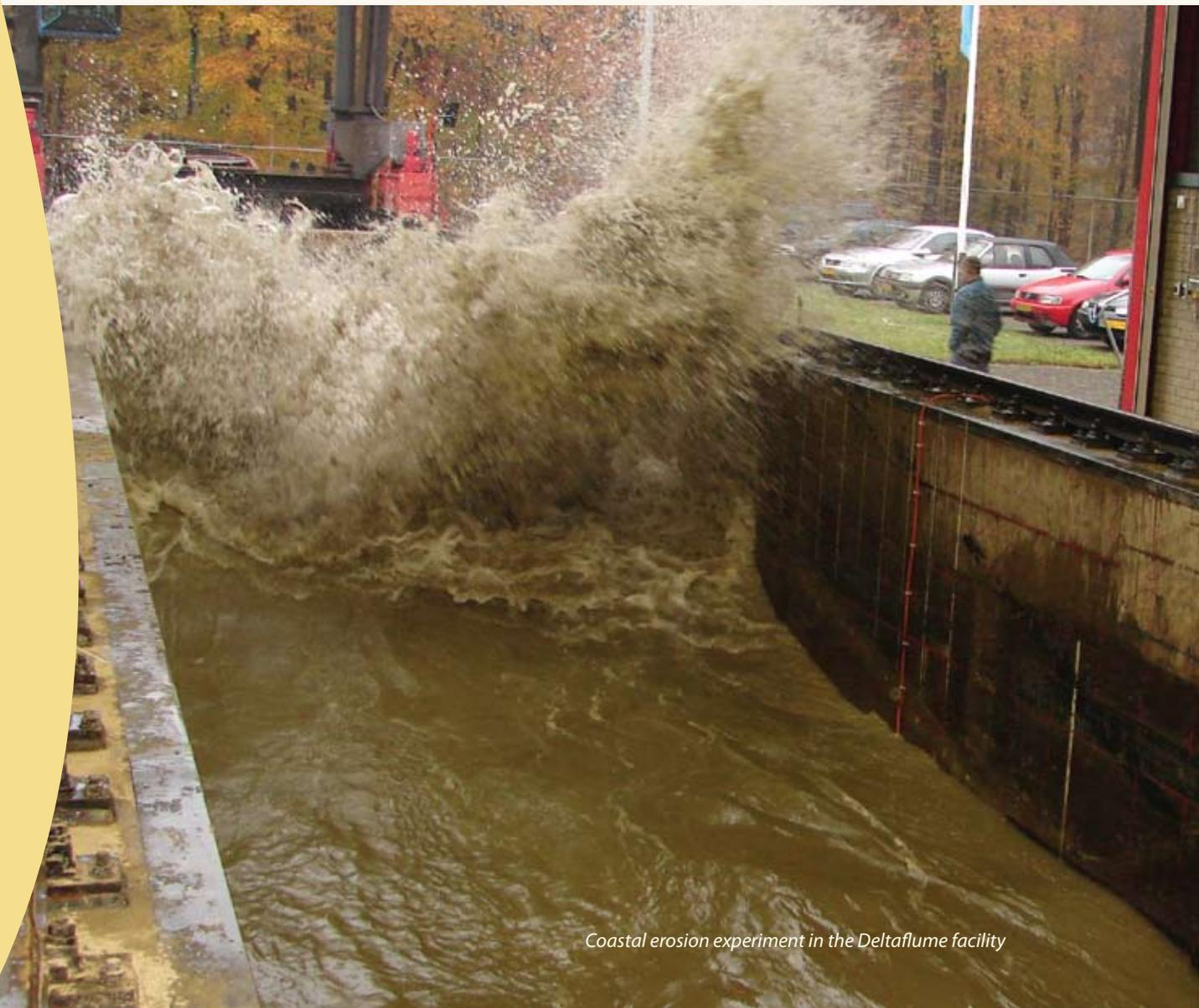
*Coastal erosion experiment in the Deltaflume facility*
